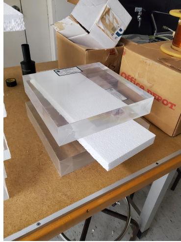
Figure 5.4: Scintillator for the two end panels, also wrapped and separated.
