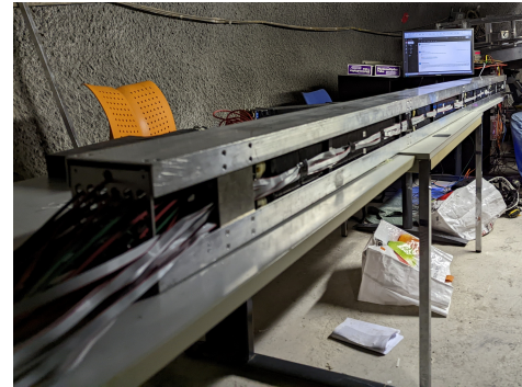
Figure 5.72: LV cables are properly taped to the sides of this supermodule, holding them in place.
