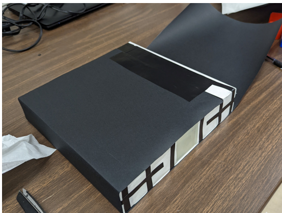
Figure 5.41: Step 4: Black paper being wrapped around Tyvek.
