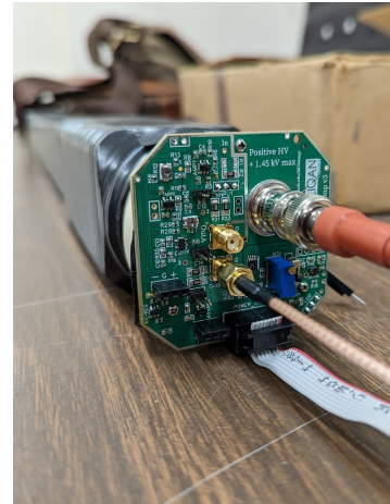
Figure 6.21: Proper cables inserted into a bar's base.
