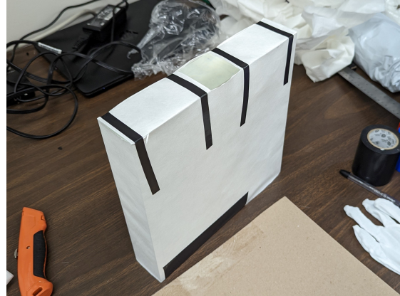
Figure 5.38: Step 3: Tyvek end caps added and secured with strips of tape.
