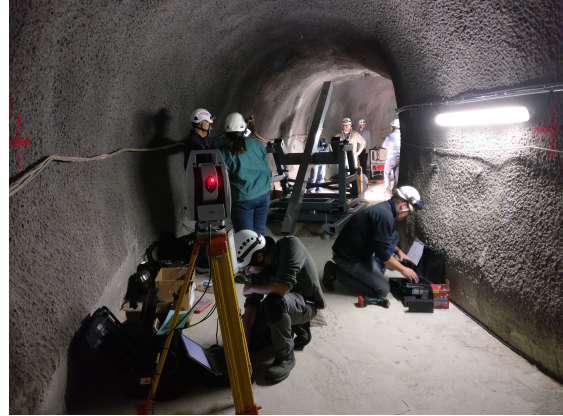
Figure 4.6: The CERN survey team working with MilliQan to align the detector's support structure toward the CMS IP using special CMS-coordinate marking devices.
