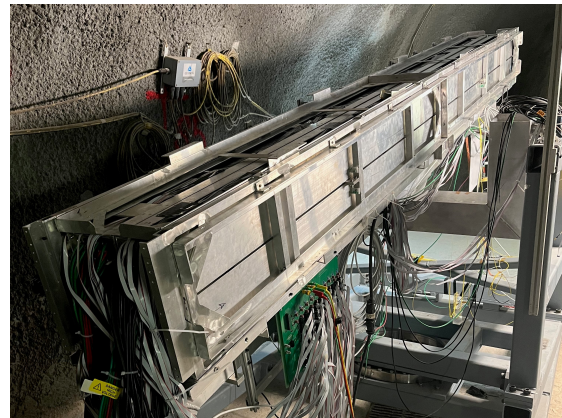
Figure 5.96: All four supermodules inserted in the detector, visible due to removed panels.
