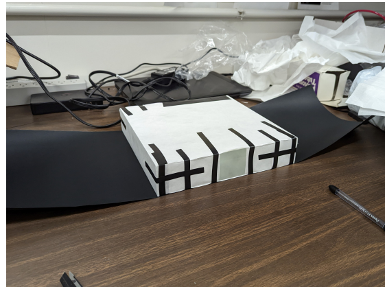
Figure 5.40: Step 4: Wrapping process begins again with black paper.
