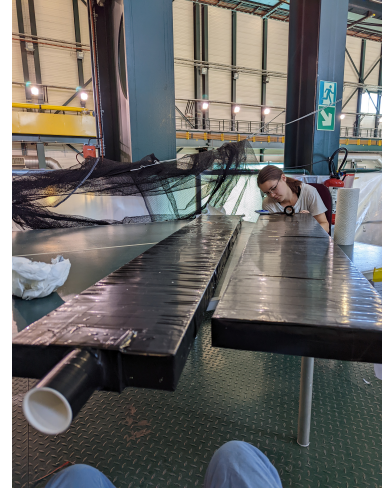
Figure 5.49: As with any other mount, these mounts are fully wrapped with black tape against the scintillator.
