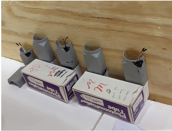
Figure 5.31: Bar mounts glued with epoxy and propped up to dry. The leads of LEDs sprout from the top, positioned so the glue sealing their insertion hole is able to dry.
