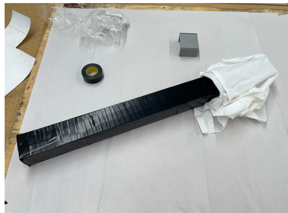
Figure 5.30: Step 8: Bar double-wrapped in tape, with the exposed end covered by cloth.
