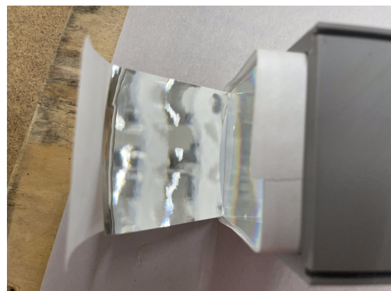
Figure 5.24: Step 6: Inserting the first strip of the end cap, not yet having tucked in one of the two sides.
