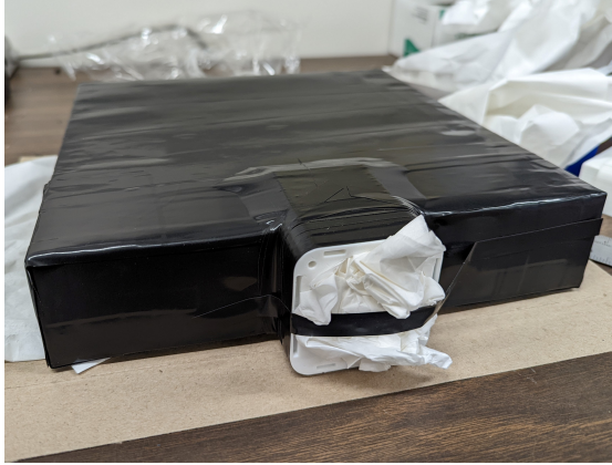
Figure 5.43: Step 5: Fully wrapped end panel, with scintillator-half of plastic PMT mount attached and wrapped.
