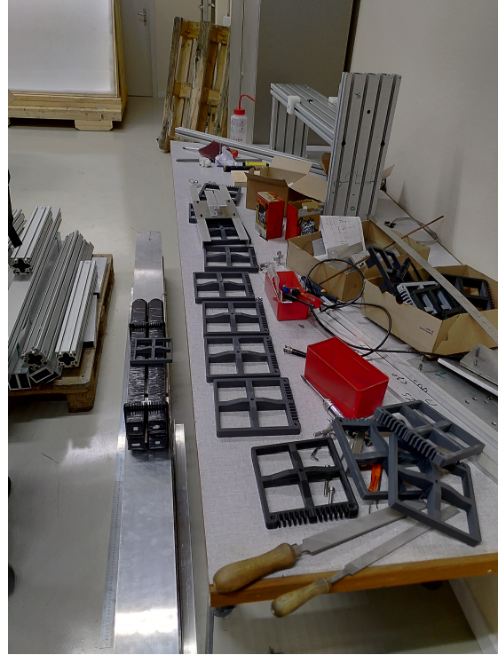
Figure 5.51: A collection of unit braces, newly printed in a CERN workshop by Robert Loos.
