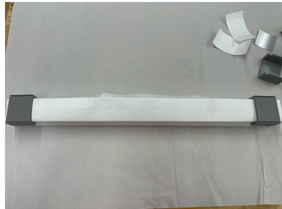
Figure 5.22: Step 5: Tyvek folded fully around bar, creased at each fold.
