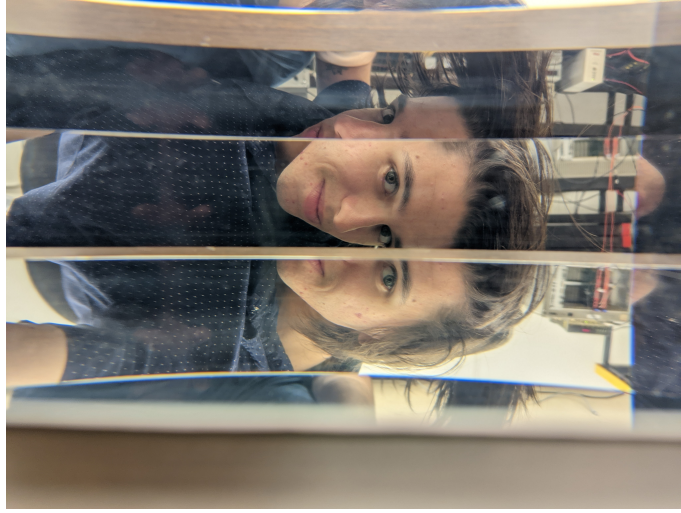
Figure 5.34: Panels also act as a light-guide, reflecting my face once again. Reflective caps are not necessary, since it is unlikely for light to make it across the panel to the PMT.
