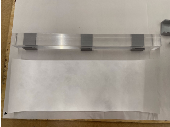
Figure 5.19: Step 2: Bar resting on creasers, ready to have plastic unwrapped.
