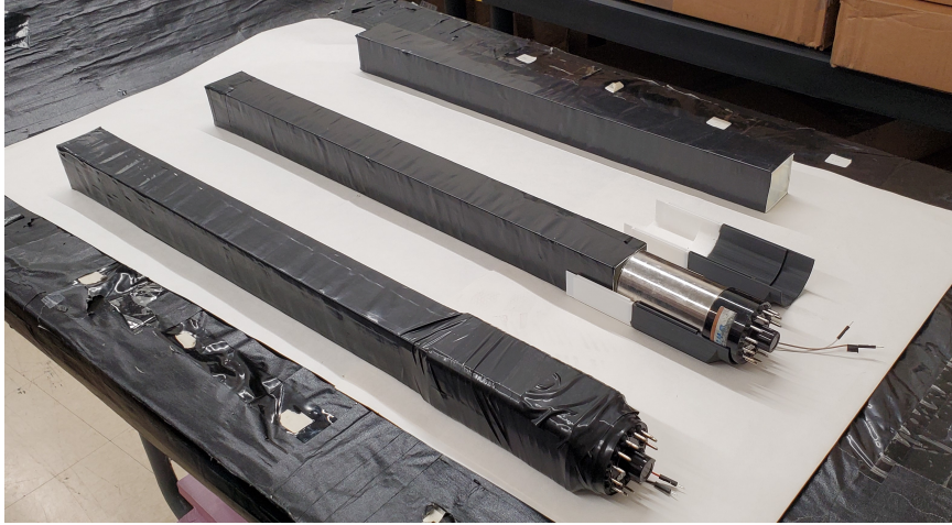
Figure 5.32: Stages of mounting a PMT. Right: Fully wrapped bar, with exposed scintillator. Middle: Two glued halves of plastic mount, one of them holding a PMT against the bar and the other lying adjacent, ready to be closed over the top. Left: Fully wrapped bar with mount and PMT attached. Leads of LED stick out next to the PMT.
