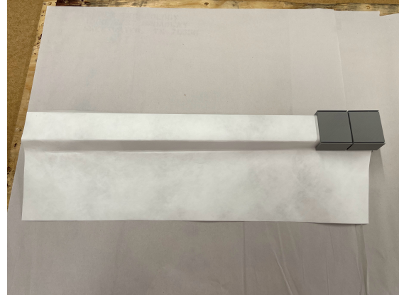
Figure 5.20: Step 3: Creasers are slid to ensure tight first fold of Tyvek over bar.
