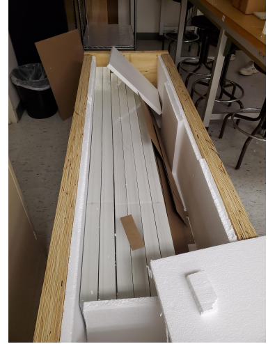
Figure 5.5: Scintillator for the six side panels, the two top panels wider than the others.
