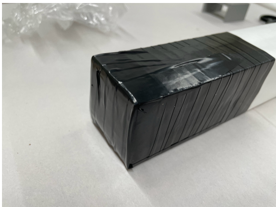
Figure 5.29: Step 7: End of bar fully wrapped in tape. This is continued over entire bar.
