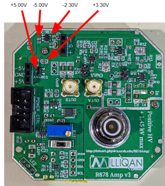
Figure 5.14: Convenient probing locations on the base board and their expected voltages, used to determine whether it is functioning correctly.
