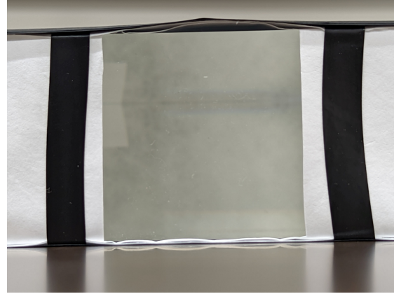
Figure 5.44: Step 6: inside of wrapped panel, as seen through square hole left open for PMT mounting.
