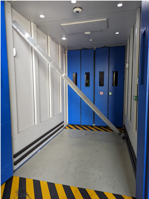
Figure 4.7: A creative experiment in transporting supermodules to the Gallery without a crane: a supermodule lid is balanced diagonally to fit in the radiation scanner required for all materials entering and exiting the CMS underground.
