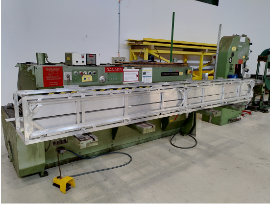
Figure 5.87: The interior of the MilliQan cage after its construction, without attachment points for panels yet added to the outside.
