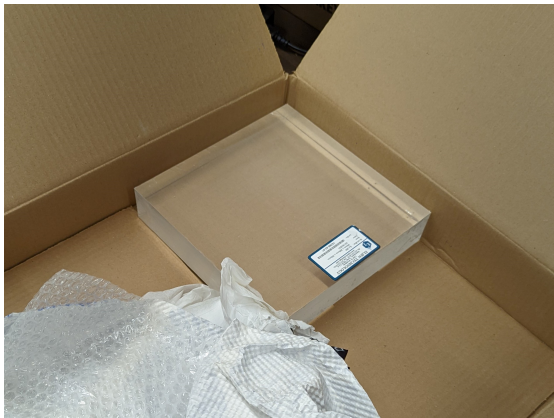
Figure 5.35: Step 1: End-panel scintillator, still wrapped in plastic. Other materials not pictured.
