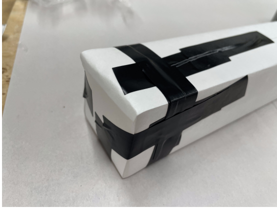
Figure 5.25: Step 6: Full end cap inserted and secured.
