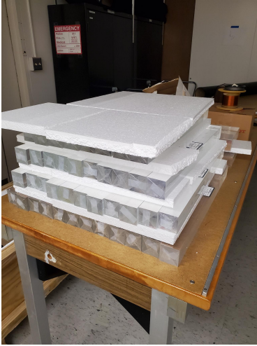
Figure 5.3: Bar scintillator, wrapped in plastic. Styrofoam spacers prevent scratching.
