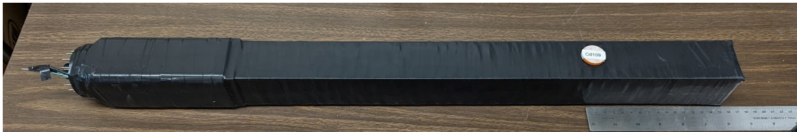
Figure 6.22: A bar sits with a small Cd-109 source puck sitting along its bulk at UCSB.
