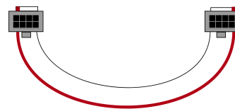
Figure 5.62: Ribbon cables in MilliQan are inverted from end-to-end, due to an inversion in the pin mapping on the power distribution board.
