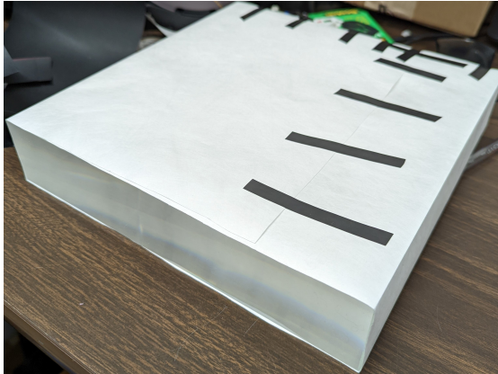
Figure 5.37: Step 2: Tyvek wrapped fully around scintillator.
