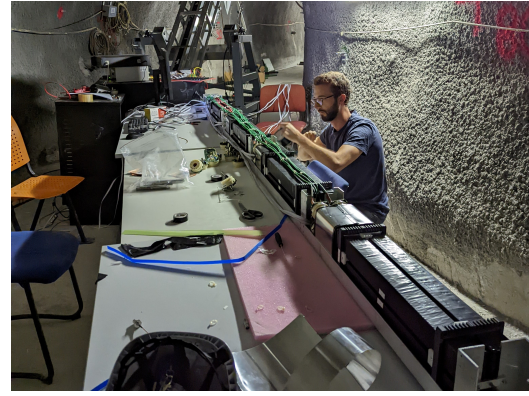
Figure 5.70: David Vannerom checks each unit in a fully cabled supermodule to ensure no LEDs or bases have come loose.
