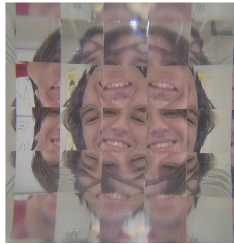
Figure 5.28: My face through a bar without an end cap, demonstrates its properties as a light-guide.
