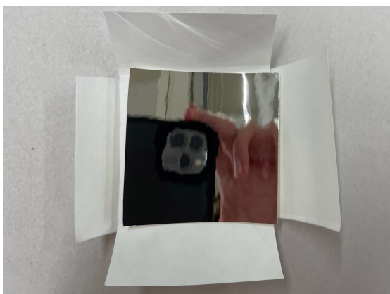
Figure 5.23: Step 6: Tyvek strips and square of reflective material, laid in the shape of an end-cap.
