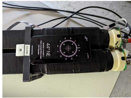
Figure 8.20: In order to measure the angle of rotation for units in this study, the built-in magnetometer of a smart phone was used.
