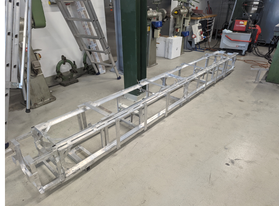
Figure 5.88: The full supermodule with all panel attachment ports, spacers, and parts used for angling the inserted supermodules.
