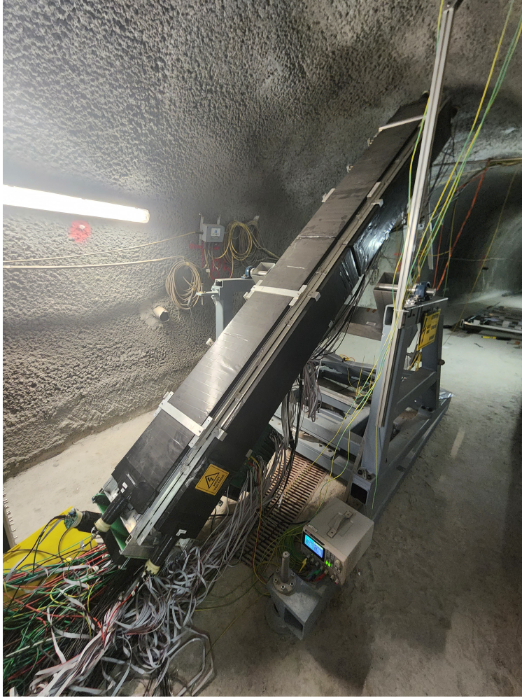
Figure 5.19: The Run 3 bar detector. One of the hardest challenges of the bar detector is cable management, as each of the 72 total scintillator channels is supplied by 3 cables, and all cables enter the detector from a similar point very close to the ground. The LV supply and LV splitter board can be seen near the bottom of the figure.
