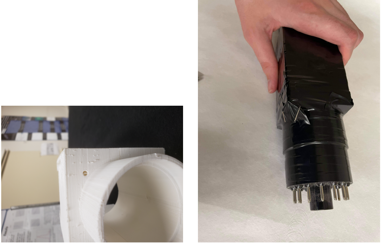
Figure 5.14: (Left) A picture of an early design of the PMT mounts. An LED hole is bored nearby the PMT, offering an LED mount for light injection. The hole is not bored fully into the PMT, providing a small amount of natural attenuation for the injected photons to aid in the production of SPE-like signals. The mount itself is porous to light so must be fully wrapped. (Right) A scintillator, PMT, and LED mounted into a fully wrapped bar.
