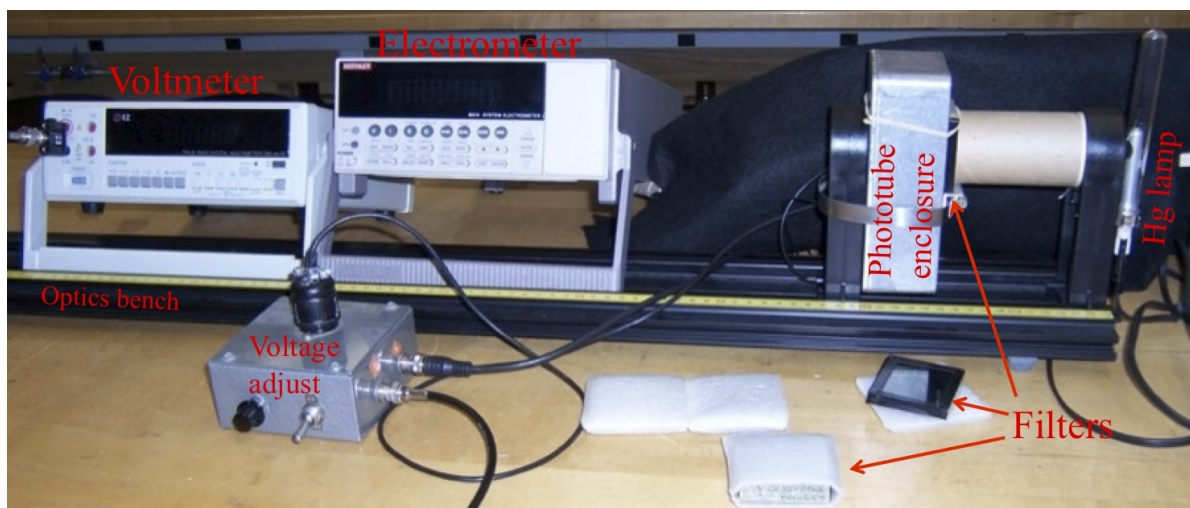
Figure 13: Photo of the apparatus mounted on an optics bench.
